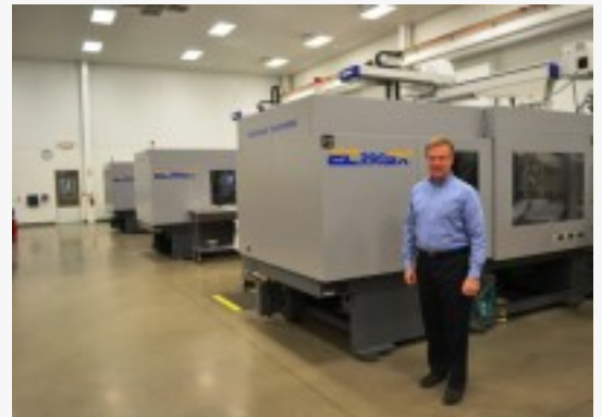
David Lennox, vice president of Operations for C&J Industries, introduces one of the new all-electric Toshiba injection molding presses.
