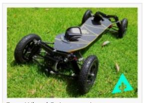
Four Wheel Drive, maximum power rating of 12kW, full suspension, jump friendly, the new BajaBoard looks to open up new possibilities on the action sports and board sports scenes.
