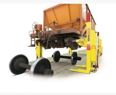
70 tonnes, meaning that the SKYLIFT has the flexibility to be used as a single long lift or two individual lifts.
