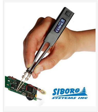
while testing the small components. LCR-Reader from Siborg Systems Inc. are the solution to these problems.
