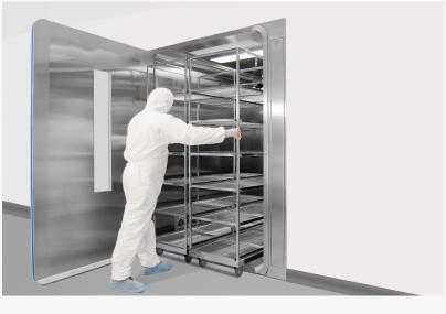
validated using a Bio-indicator (BI) Challenge. The 2 hour cycle duration is inclusive of aeration down to a level of <2ppm H2O2 while working independently to the facility's HVAC system.
