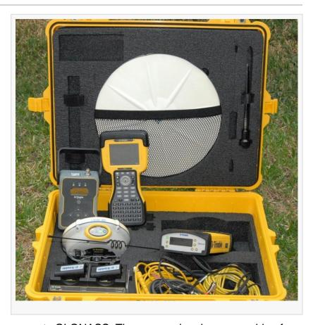
Modernization signals, L2C and L5. It also supports GLONASS. These new signals are capable of providing surveying professionals with real field benefits.
