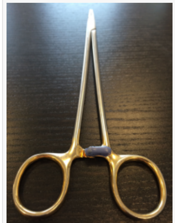
Xerafy RFID UHF tag attached to the surgical instrument. With UHF technology, it is possible to get a good read range from many tags simultaneously
