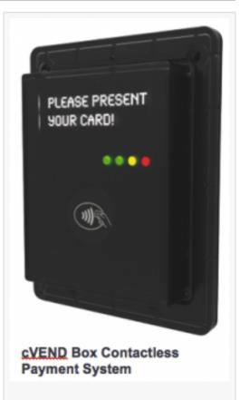
cVEND is available in three variants, including cVEND plug, which can be integrated into validation terminals almost invisibly, and cVEND box, which can be mounted in any kind of metallic kiosk-type systems, terminals and ticket gates, either with or without a display.
