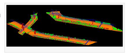
Airborne LiDAR(Light Detection and Ranging) widely used technology for Power line Mapping due to its data efficiency and cost-effective outputs. The Georeferenced LiDAR data is extremely useful to get the terrain, tower location, tower structure, power line catenary models, and vegetation.
