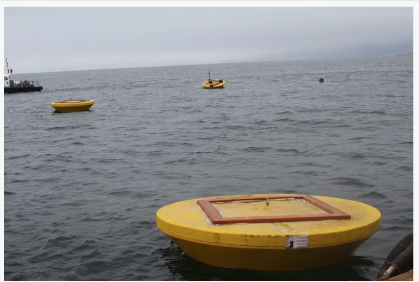
With small individual size, a full array of 15 pumps can deliver ~225,000 cubic meters of fresh water annually.
