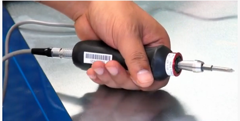
SDX torque sensor is an instrument designed for torque auditing, verification or tightening fasteners.
