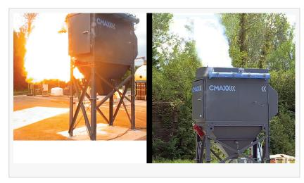
There was no trace of flame or spark transmission downstream of the IDA filters or in the clean air plenum.
