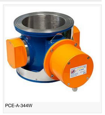
Suitable for the continuous monitoring of dissolved substances or suspended solids in wastewater, the PCE-A-344W in-process sludge consistency meter uses microwaves to penetrate the surface of the sludge every second and obtain consistency readings without heating. An integrated temperature probe ensures the readings are accurate from 5°C to 50°C (41°F to 122°F).
