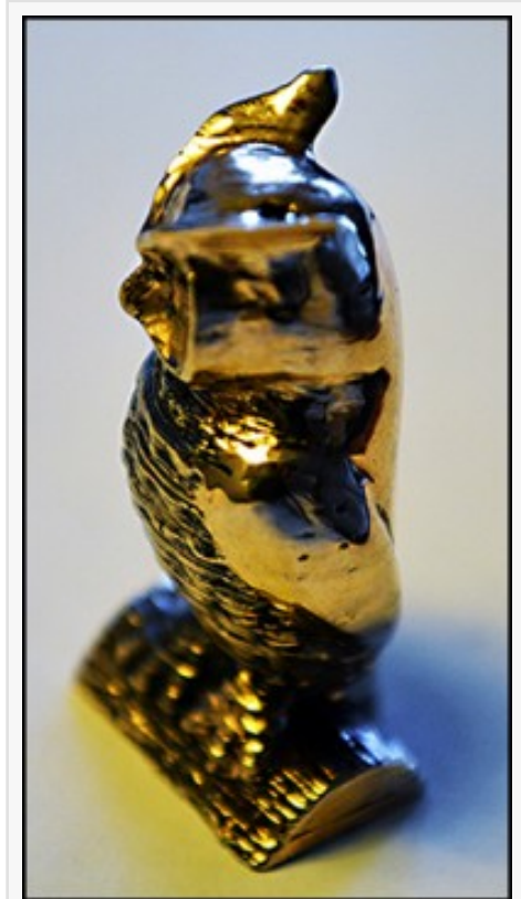
Owl printed in Filamet™ Bronze with a sub $1000 3D Printer.
