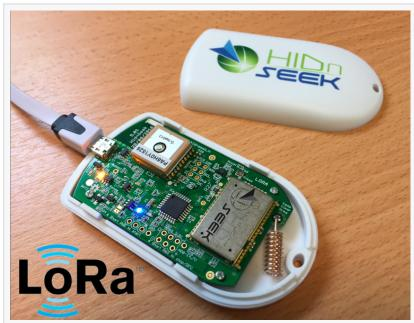
Powered by Microchip RN2483 - LoRa® Modem Long-Range, Low-Power Wireless Solution
