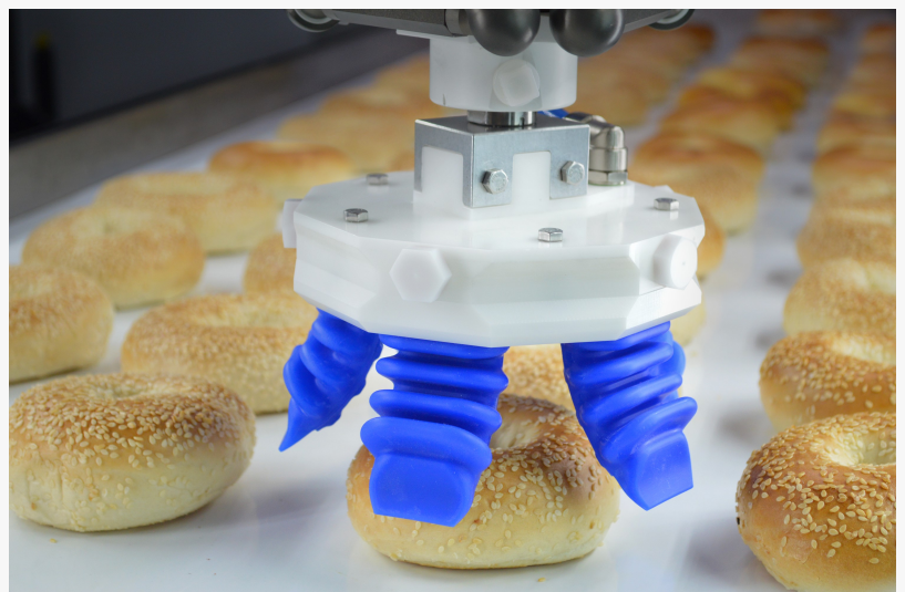
Soft Robotics Enabled Bagel Handling
