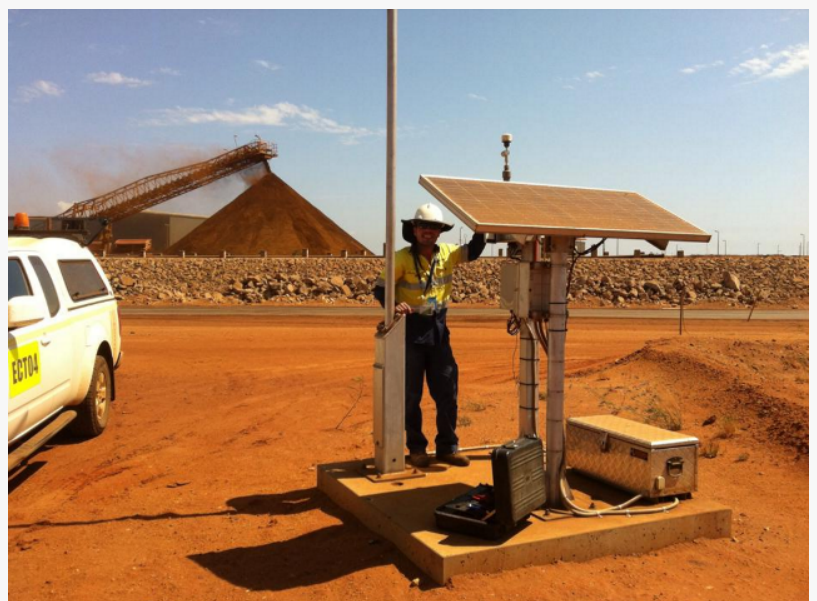
Solar powered particulate monitor on a mine site in Western Australia.
