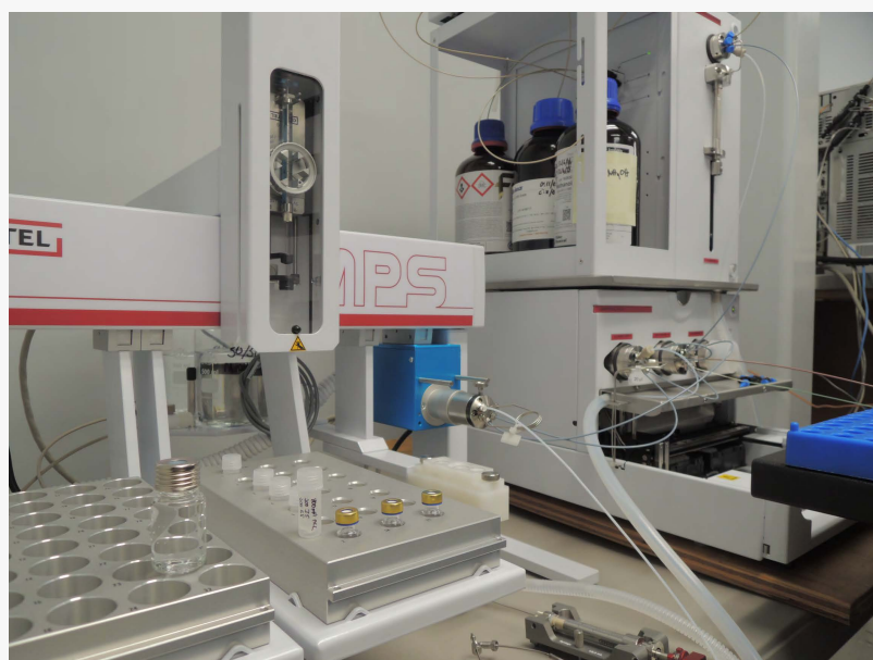
PFAS MobiLab uses state of the art solid phase extraction and liquid chromatography to confidently identify and quantify PFAS in water and soil matrices
