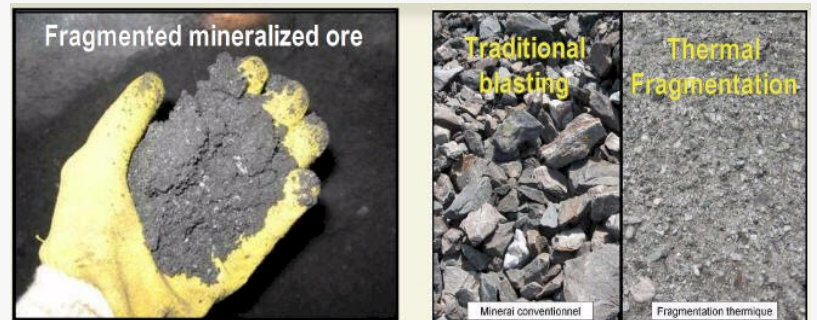
Spalling/crushing of rock to 0 to 13 mm, More efficient & less expensive
