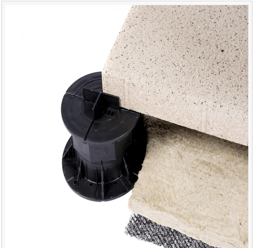
The SpongePaver™ System incorporates the needed mineral hydro blanket with a drainage mat under a traditional paver to help control runoff under rooftop patios, walkways and fire-free zones.
