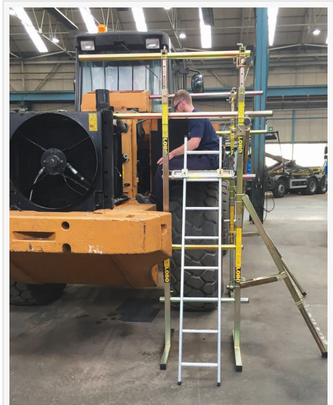
Plant maintenance work platform
