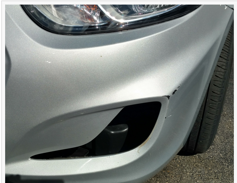
Driving light missing from vehicle. Possible safety, legal, and financial liability.
