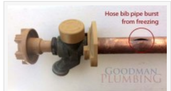
Asheville plumbers repair outdoor spigot pipe burst from leaving hose on in freezing temperatures
