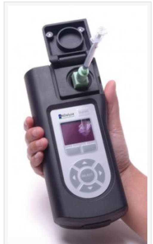
ANDalyze AND1100 instrument and DNA enzyme sensor for testing lead in drinking water within US EPA limits
