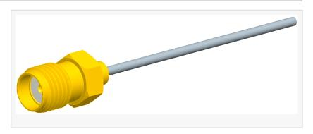
features high-performance 0.047 and 0.085-inch diameter hand formable semi-rigid cables. The cable assemblies feature a gold plated, precision machined brass body, a gold-plated beryllium copper contact, and PTFE insulator.
