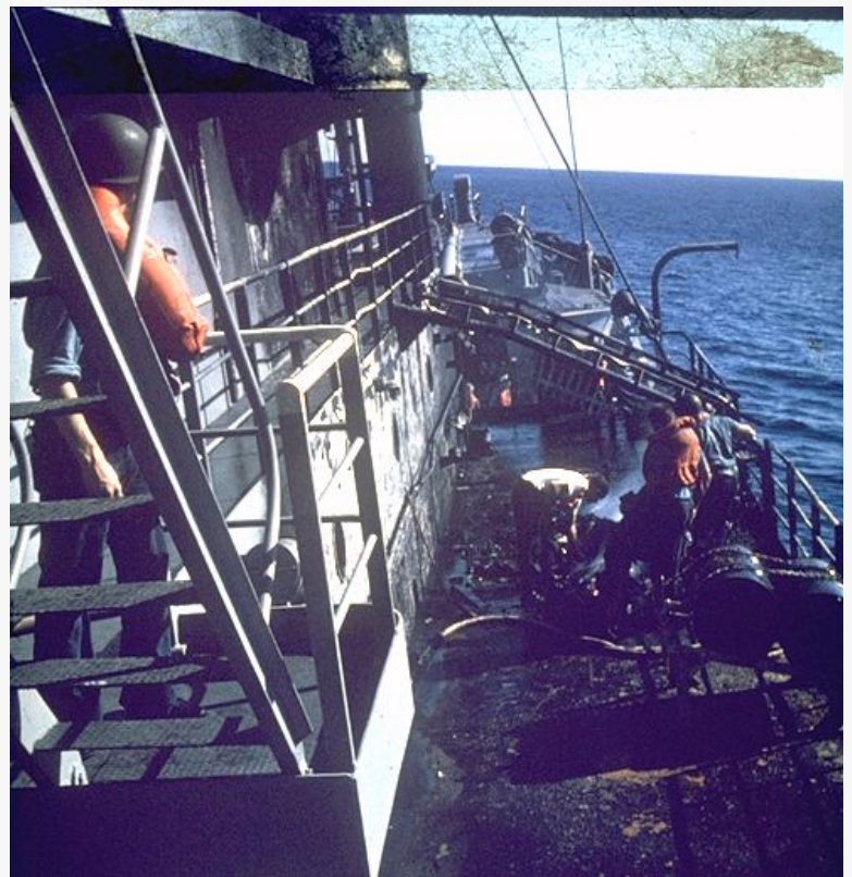
(photo: USS Liberty Memorial) USS Liberty Starboard Napalm Damage -- This photo shows napalm damage to the starboard side of the superstructure and deck.
