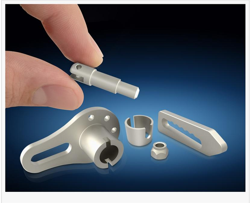
TiMIM part features can include undercuts, varying wall thickness up to .125" or 3mm. TiMIM parts also accept many surface finishes including anodizing and electro polishing and can be finish machined if necessary.
