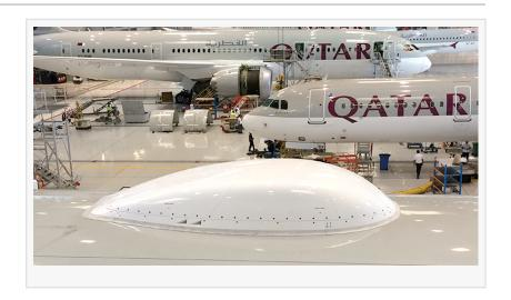
Working directly with Inmarsat, EAD Aerospace developed the complete solution, produced the engineering package and received the STC within a tight timeframe, allowing the end customer, Qatar Airways, to begin the installations around regular maintenance inputs.
