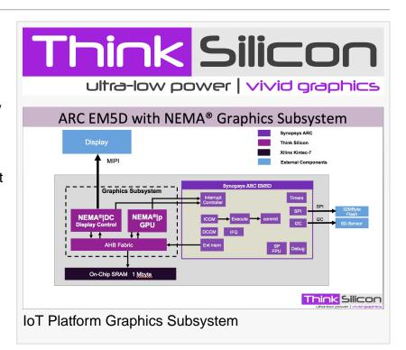
The prototype combines the best of Synopsys technology sporting a DesignWare® ARC EM5D Processor with Think Silicon products including NEMA|p, NEMA|DC, and NEMA|GFX-API, resulting in a developer solution aimed at ultra-low power connected wearables and low-power embedded applications. Both companies have tools to assist developers in creating world-class products for a
