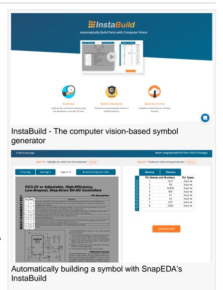
The symbols are automatically mapped to verified IPC-compliant footprints. The designer can then download the ready-to-use symbol and footprint for their desired PCB design software.
