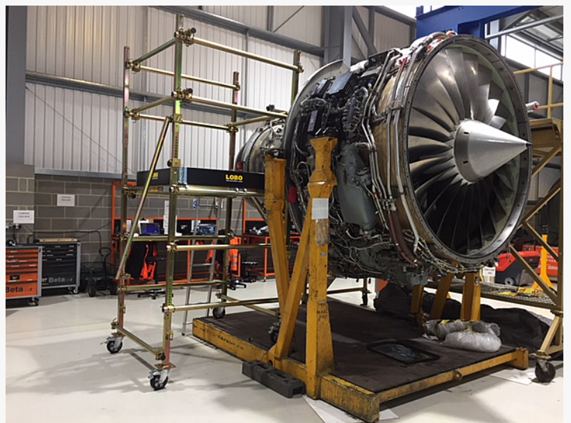
Split level work platform
