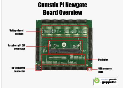
This board lays out every feature of the Raspberry Pi® Compute Module and Compute Module 3. Easily monitor digital, analog, and differential signals via 0.1"-pitch pins.
