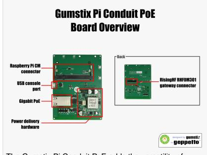
The Gumstix Pi Conduit PoE adds the versatility of power-over-Ethernet to your LoRa gateway.
