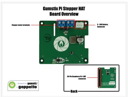
Provides rotational accuracy below a tenth of a degree by way of the TI DRV8846, a 4 - 18V, 1.4A stepper motor driver.
