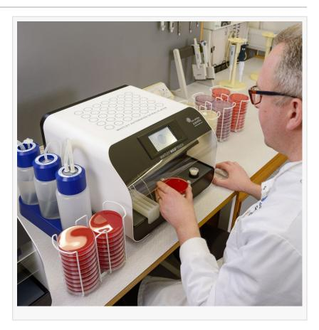
increased quality control measures have led to laboratories looking more to automation to help improve reproducibility and accuracy. Spiral plating offers a real reduction in the cost-per-test and standardises counting methods. Serial dilutions, for many users, can be eliminated, which in turn saves time, the cost of consumables and space in the incubator.
