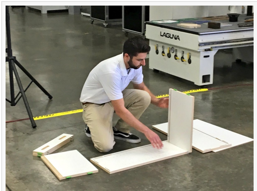
Lockdowel Engineer Daniel Savage demonstrates glue-less, snap-together assembly for furniture, cabinets and closets.
