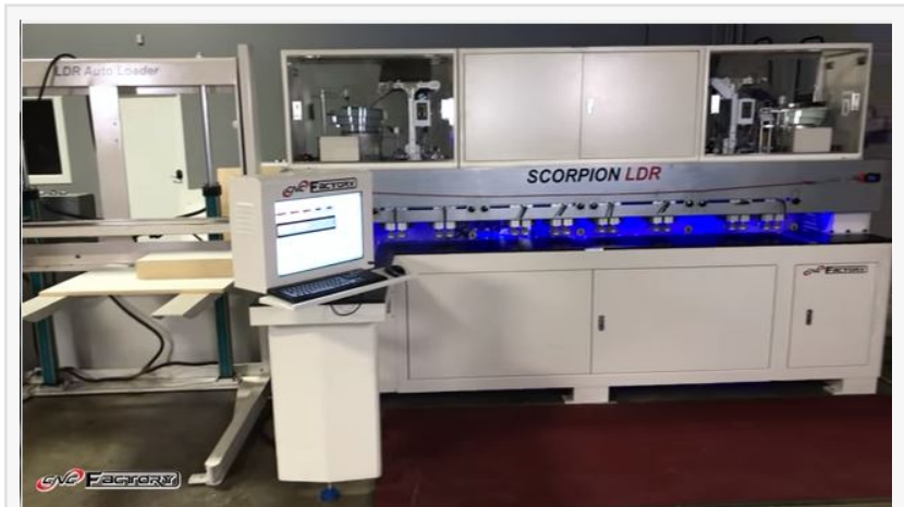
The Lockdowel Scorpion LDR inserts glue-less Lockdowel fasteners and allows super fast assembly of furniture and cabinets.
