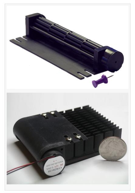
and scientific instruments as well as portable electronics. The X series offers four models measured in length of its air outlet from 1"(25.4mm) to 4"(101.6mm) with unique height of 23mm. With the builtin tachometer sensor, the speed of the X series can be controlled by regulating 5VDC or 12VDC. It also can be controlled by PWM. The full ball bearing system supports motor continuously running life expectancy greater than 65K hours with RoHS compliance.
