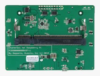
Add power and multiple features with the Chatterbox Pi such as as 15-pin CSI 2 camera connector, RGB LED, WiFi, and Bluetooth, as well as a 20-pin GPIO header to RPi CM devices...
