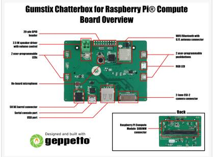
The Chatterbox Pi comes ready to use for prototyping or designers can easily copy and modify the board design in Geppetto® D2O to create their own custom Raspberry Pi CM based AVS or IoT design in minutes.
