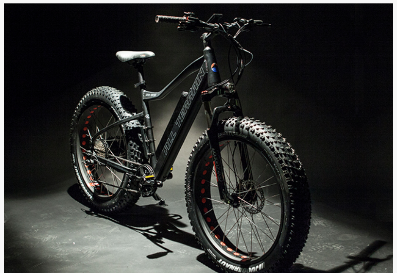
The All Terrain R500 features 4" tires, a powerful 500 watt rear hub motor and long-range battery.
