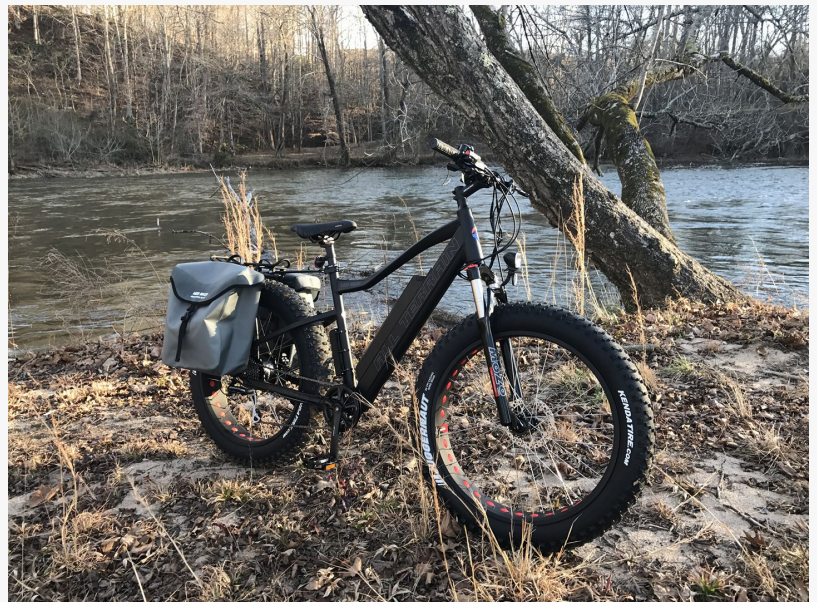
The All Terrain R500 features 4" tires, a powerful 500 watt rear hub motor and long-range battery.
