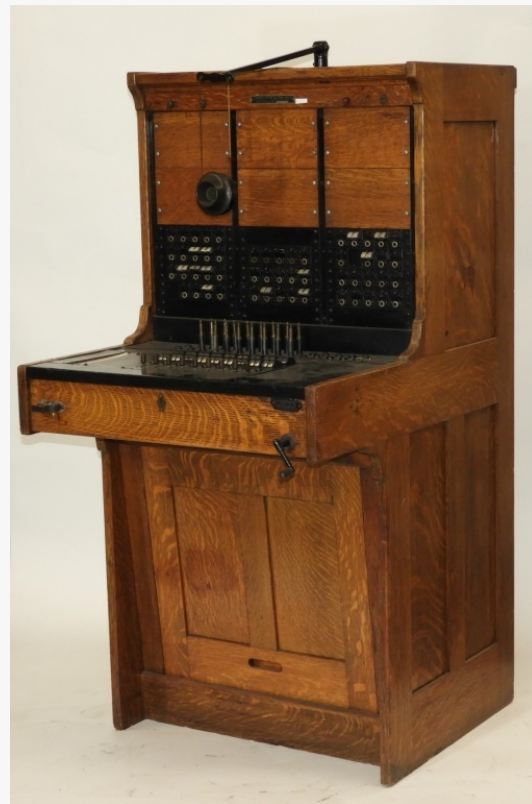
Early 20th century Stromberg & Carlson telephone operator switchboard, in an oak case.
