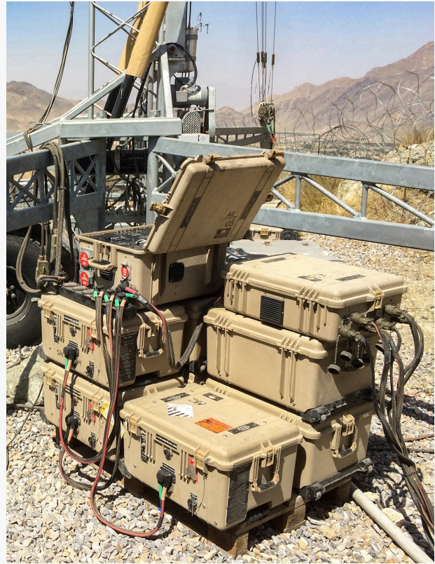
An Alternative Energy System (AES) is shown deployed with a Persistent Surveillance System-Ground (PSS-G) tower on a mountaintop in Afghanistan.
