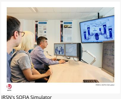
The FA3 simulator is one of four PWR simulator configurations that can be operated on the Simulateur d'Observation du Fonctionnement Incidentel et Accidentel (SOFIA). The current
