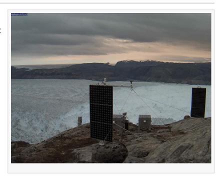
charge the batteries and power-up the system remotely. The goal of the experiment is survival of the batteries for 6 months at a [0%] state of charge, K2 Energy is confident that the batteries will be able to continue balancing, charging, and powering this system autonomously for even longer.
