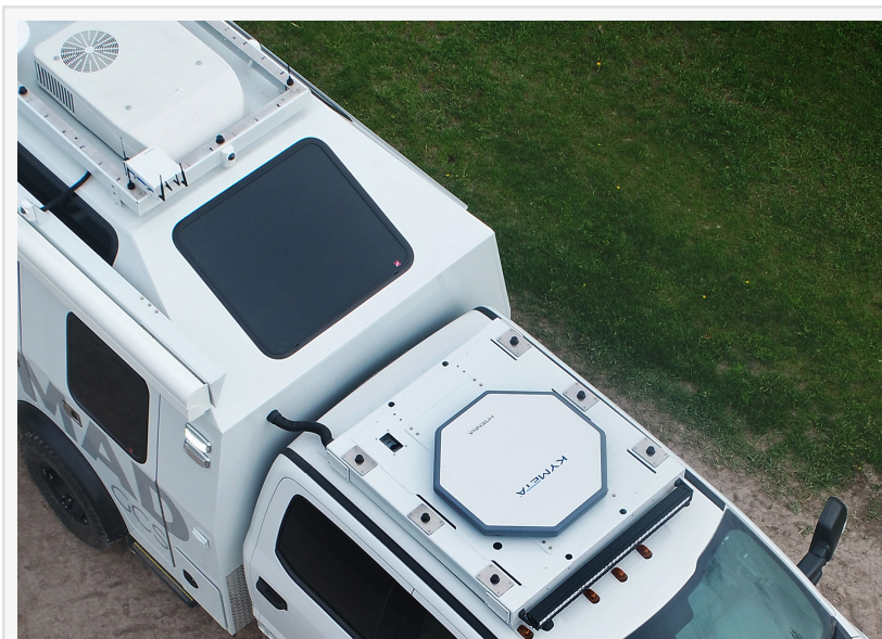
Kymeta electronically-steered, flat-panel antenna on top of the emergency response vehicle
