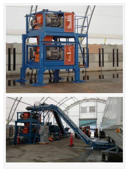
chips into precision, flowable particles down to 1mm size for producing energy pellets, biochemicals, biofuels, and other bioproducts. The Crumbler® P24M-150e-2 is unique in that it processes high-moisture feedstocks using very low energy and without the need to pre-dry the biomass. The Crumbler® system is installed and processing wood chips into 6mm particles at Proton Power's renewable diesel plant in Rockwood, TN.
