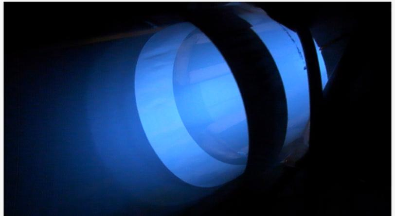
Airbreathing ion-propulsion engine breadboard from SpaceLab EU
