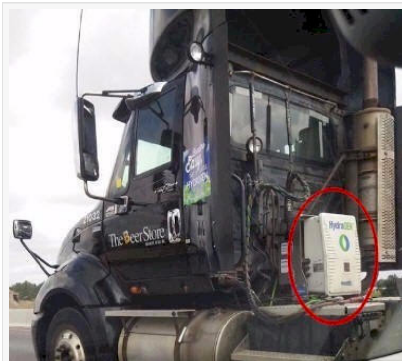
dynaCERT HG1 unit installed on diesel Truck
