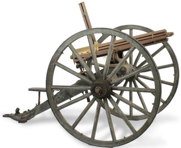
Colt Manufacturing Company Model 1875 Gatling Gun, .45 caliber and marked "NJ".
