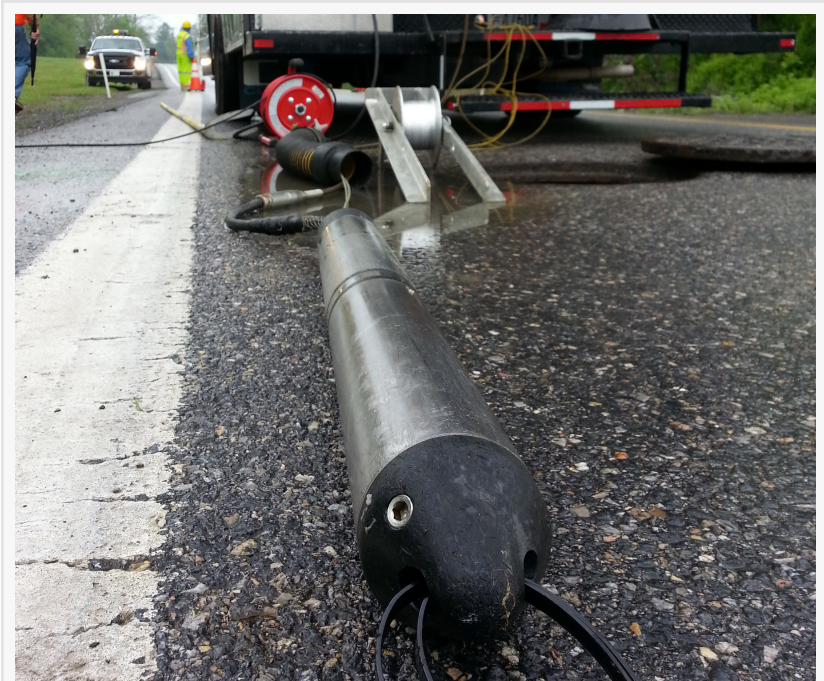
Electro Scan's Rugged, Machine-Intelligent Assessment Probe Precisely Locates Pipeline Defects and Quantifies Leakage Rates in Gallons per Minute or Liters per Second.
