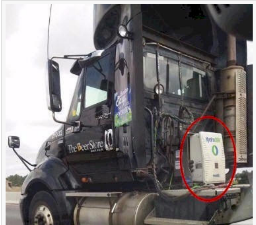
dynaCERT Smart-ECU controlled HG unit installed on diesel Truck
