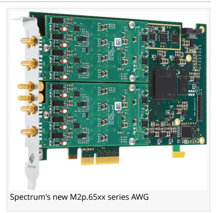
outputs, these latest cards will be of interest to all the engineers needing signal generators for frequencies between 1 and 60 MHz in the areas of ultrasound, laser, LIDAR, radar, automotive, medical science and big physics experiments.
